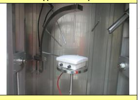
3. Test for protection against solid foreign objects (Dust test)
