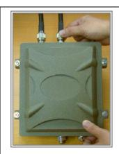
Most of the problems of outdoor models are from the connector connections that loosen over time due to vibration or other forces, even allowing moisture to penetrate the connector and seriously affecting the data and radio signal transmit. The following recommendation is used for all outdoor installation to be waterproofed.
