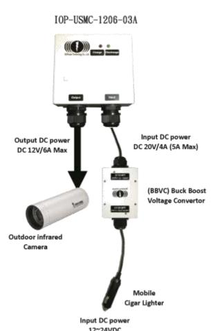
IOP-USMC-12V0206-II series is specifically designed for large power equipment vehicle load system, through vehicle cigarette lighter-powered uninterruptible operation of the system, such as on-board infrared camera, car video host, DVR/NVR 12 hour record, the range of temporary large discharge current device must be over 12 hours or longer-lasting forms online without interrupting the operation of the power system.
