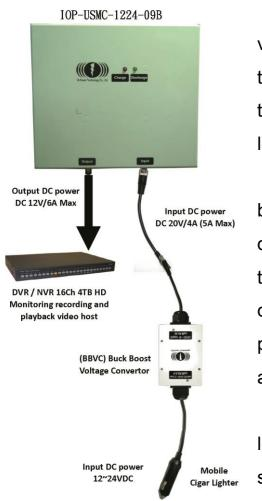
IOP-USMC-12V1224-OA series is specifically designed for large power equipment vehicle load system, through vehicle cigarette lighter-powered uninterruptible operation of the system, such as on-board infrared camera, car video host, DVR/NVR 48 hour record, the range of temporary large discharge current device must be over 48 hours or longer-lasting forms online without interrupting the operation of the power system.
