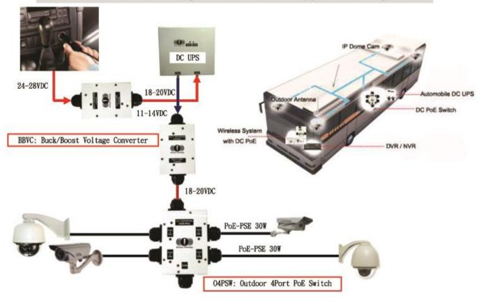
BBVC - Buck / Boost Voltage Converter Multi-application Diagrams 02
