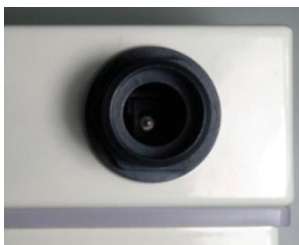
DC Jack Female (inserting DC Jack Male)
