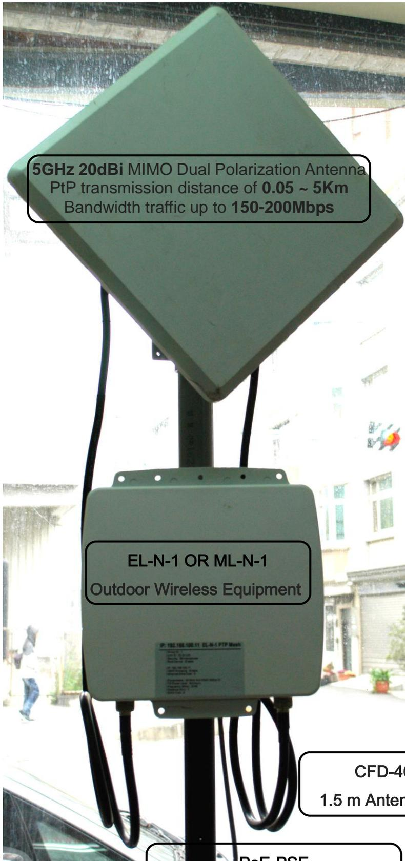
5GHz 20dBi MIMO Dual Polarization Antenna
