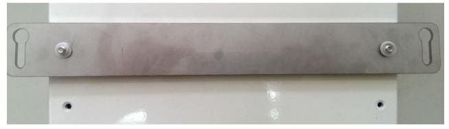
Finally, screw the bracket tight into the screw holes in the bottom side of the housing
