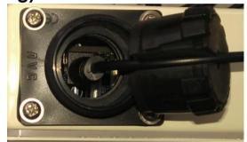
Insert the DC Jack Male head-end and into a waterproof rubber at the PCBA Female hole.
