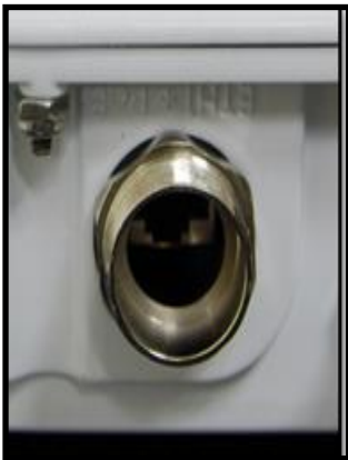
The bottom of the wireless device POE Ethernet waterproof port
