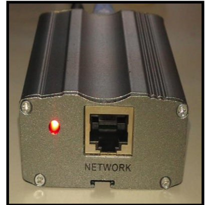
PoE Ethernet integration RJ-45 Ethernet port, connect to computer (or LAN, Camera and ADSL series with other wireless devices...)
