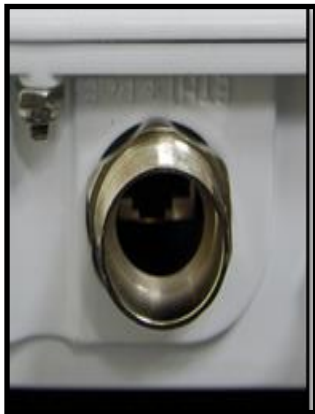
The bottom of the wireless device POE Ethernet waterproof port
