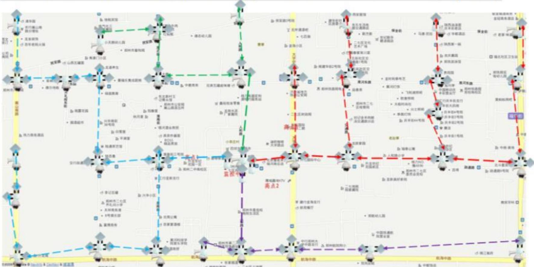
Wireless systems design guide: 1. design of multiple hops relay platform to not more than 6 jumped 2. The basis for the design, each wireless backbone links to no bandwidth over 60Mbps for design requirements 3. In the erection of three forks or crossroads, 103R three wireless module designs, reserved engineering change link direction to set up or increase future links to expand or equipment upgrade needs.
